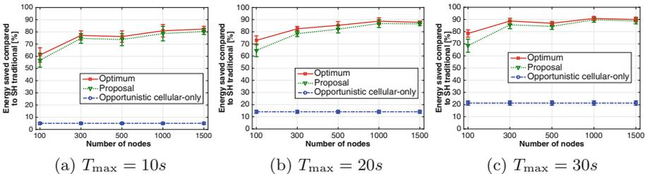
Fig. 3. Energy consumption compared to traditional single-hop.
